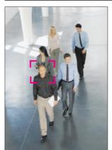
This function outputs an alarm whenever movement is detected within a pre-specified area of the image. It can also be used to automatically track a moving object or person for about 30 seconds.
